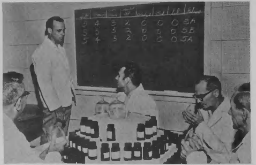
THE ODOR panel grades oil product odors at the Baytown refinery. The panel moderator stands at the blackboard and records the product ratings as called out by each sniffer.
